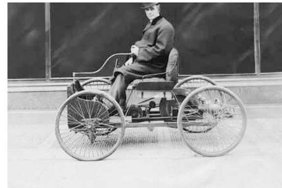
Henry Ford posing on his first automobile, the five-hundred-pound quadricycle, rolled out in June 1896. The small engine, which drove the rear wheels, is mounted behind the seat.
